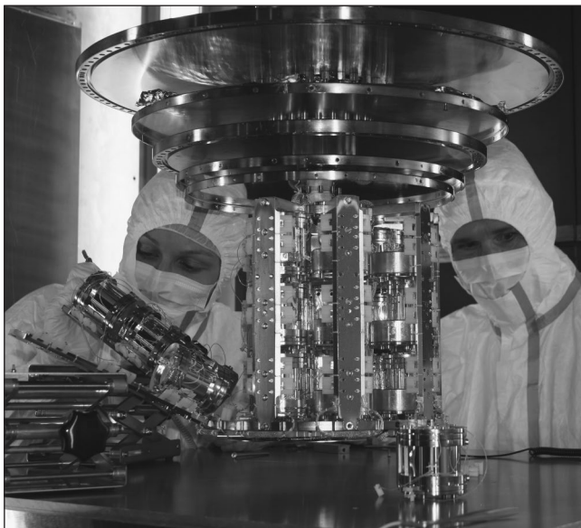
Left: A detector structure that will be used to detect dark matter particles. Each individual cylindrical detector has a \text{CaWO}_4 single crystal, similar to that shown on the bottom right. These crystals are called scintillators, and convert high-energy radiation into light. The Czochralski technique is used to grow the crystal shown on top right, which is a \text{CaWO}_4 ingot. The detector crystal is cut from this ingot.
