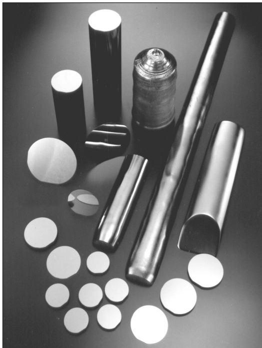
Left: GaAs ingots and wafers. GaAs is a III–V compound semiconductor because Ga and As are from Groups III and V, respectively. Right: An \text{In}_x\text{Ga}_{1-x}\text{As} (a III–V compound semiconductor)-based photodetector.
